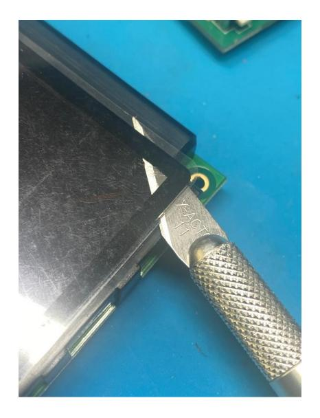
Once removed, carefully take the new screen cover and place it as accurately as possible since it will need to fit back into the chassis.
