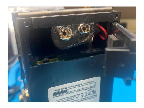
Carefully lift the leads from the battery compartment to lift the LCD board
